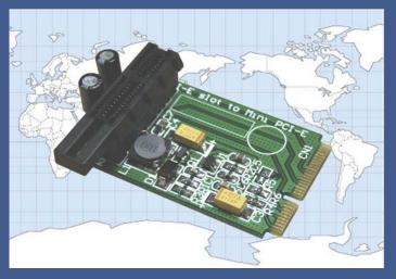
The PCI-E 1x to Mini PCI-E Card 1.0 is a debug tool for PCI-E interface card.
