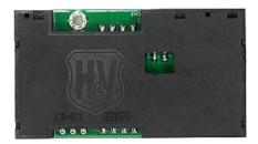
Top: USB Horizontal Connector & Controller IC
