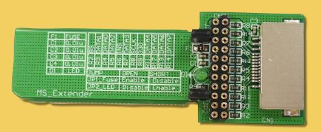
The MS Extender 1.0 is a debug and signal detection tool for Memory Stick and M2 card. It allows a Memory Stick card to be extended from the host slot for full access to the 14-pin interface.
