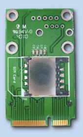
The MM2U-S half to full mini card is a converter tool for minicard interface.
